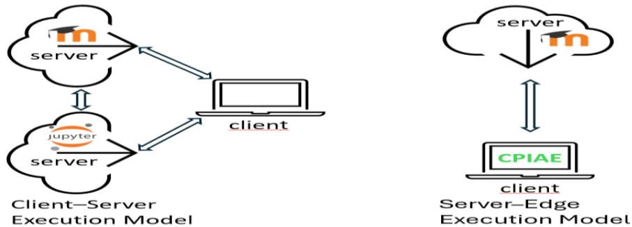
Fig. 1. Traditional client-server execution model versus the CPIAE server-edge model. In CPIAE, all Python execution occurs locally in the student’s browser.
